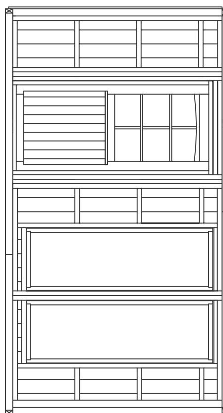
Fix wall element EL-5 with front wall elements with screws 5,0x120 together
