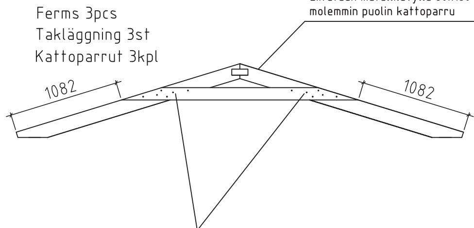
Connect with nails 4x100 (6+6) on both sides of the ferm
