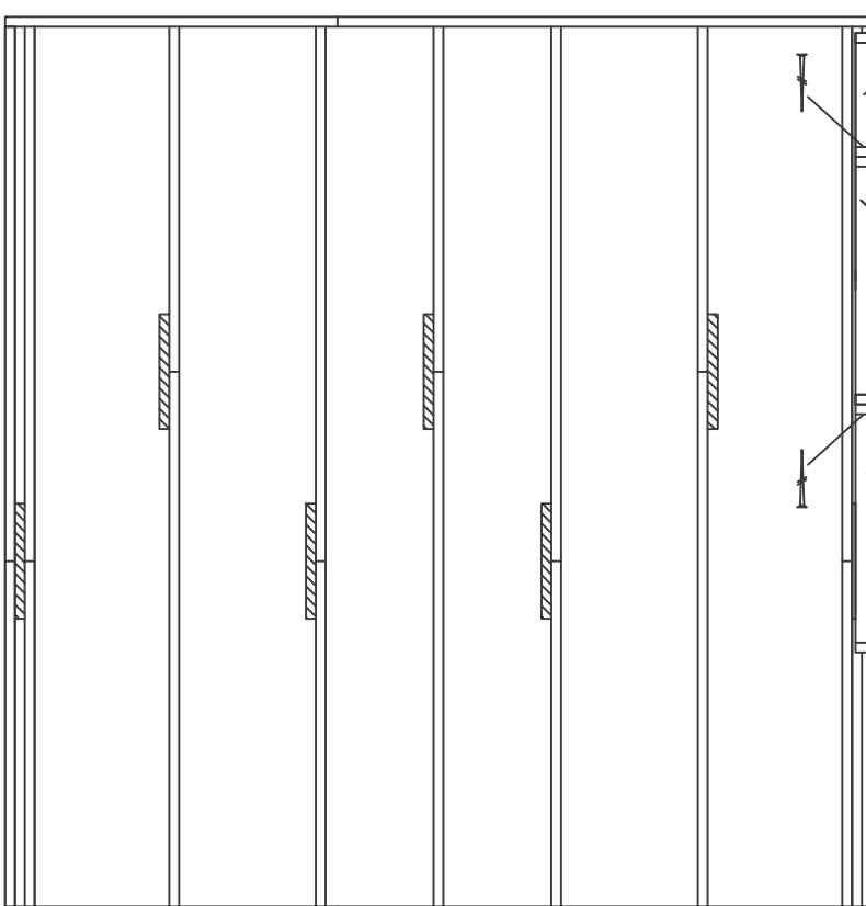
Fix wall element EL-3 with screws
