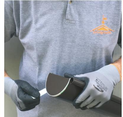
A special silicone adhesive band is already applied to the end-cap, in this way it is strongly connected to the gutter and ensures excellent sealing from the very beginning.
